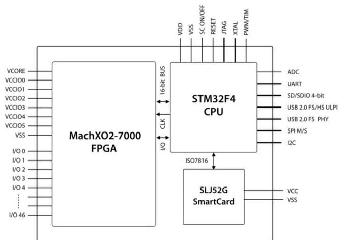
Fig. 2 SEcube Hardware Architecture
